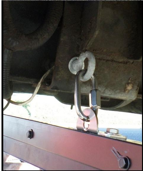
This image shows a revised hanging configuration that may be used if needed to shorten the hanging length of the mud flap. Please note that this configuration does not leave as much swing capability if a road hazard is encountered, and when lowering your coach for parking.
