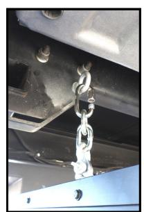
Quick link with collar screwing downward.
