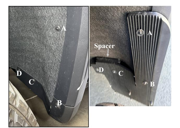
GF12 24 AT4X, GF14 24 AT4X; 2 Plastic spacers
