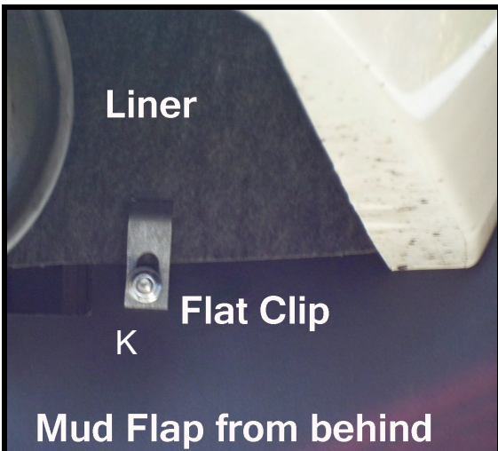
CR12 15 Tahoe and Yukon 1500 - 6 lug pattern. 2-flat clips #10001 ; 2-Plastic Spacer Brackets #10050
