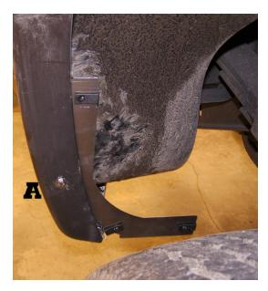
Shows how the bracket will slip behind the fender well lip. Then thread the SS Bolt thru the washer, mudflap, hole A, and then the u-clip on the bracket.
